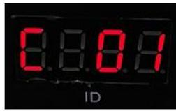
Note: When the controller is numbered, the level networking ports must be connected in strict accordance with the controller silkscreen prompt (IN/OUT); the maximum number is 60.
