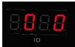
3. During the numbering process, the controller detects the number of controllers (the number of connected controllers), and displays: as shown in Figure C003, a total of three controllers are detected.
