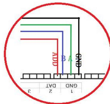
③. DMX512 single line signal line wiring diagram
