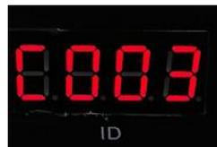
4. After completing the numbering, the first controller displays: As shown in Fig. 03 03, the first two digits 03 indicate that a total of three controllers have completed the numbering; the last two digits of 03 indicate that the last controller number is number 3.
