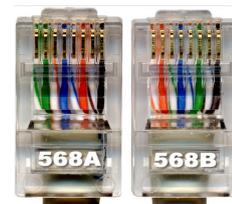
Controller and offline master controller and switch these three devices between each other using a crossover cable is better , One head is 568B, the other head is 568A. Above any equipment and computer room with a straight line , that is both 568B or 568A , Do not define the order of the straight line.
