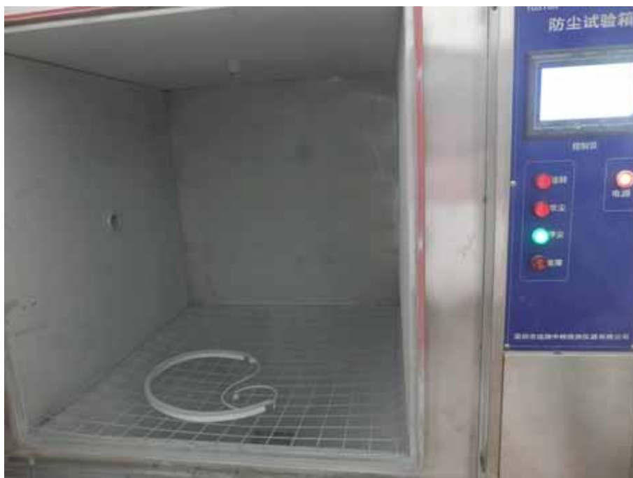
Photo 2 IP 6X TEST
