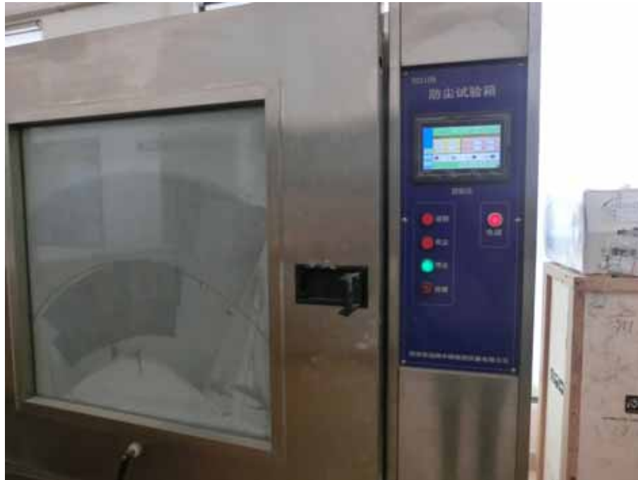
Photo 1 IP 6X TEST
