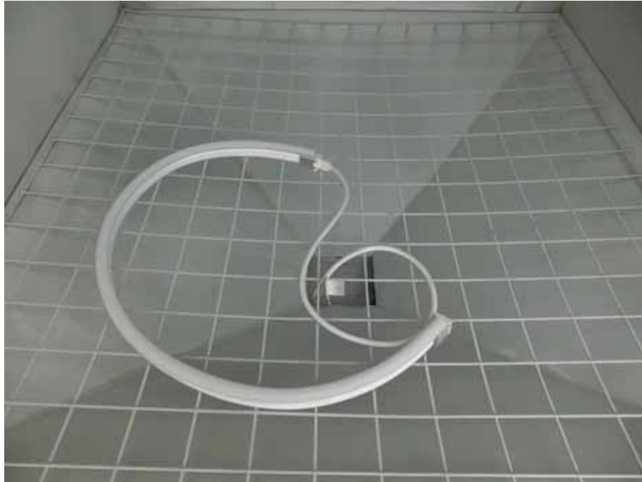
Photo 3 IP 6X TEST
